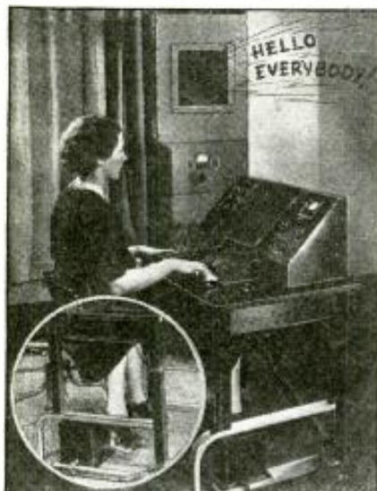
Seated at the keyboard of the Voder this young lady can carry on a conversation by pressing keys.
