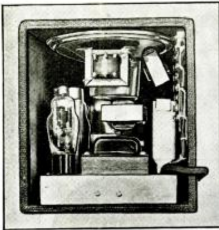
Fig. D View looking inside the cabinet. Note how compactly everything is mounted and how snugly the speaker fits in among the other components.
